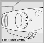
To set "Fast Freeze" ON, press the switch to "I" This switch activates intensive cooling to ensure that required temperatures are reached quickly.
